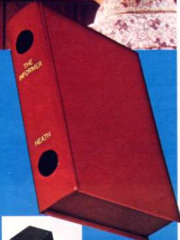
Book cover leaves rear panel exposed for access to switches and outlets. Unit can also be used without cover.
